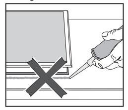
The cooktop must not be permanently sealed into the countertop when installed. The sealing strip under the edge of the cooktop provides a sufficient enough seal.
